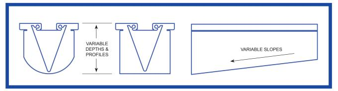
MHD's EPS foam former design flexibility allows the designer to select various system slopes, depths and section profiles to meet their specific requirements, site restrictions and hydraulics.
