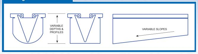
**MHD-A's** EPS foam former design flexibility allows the designer to select various system slopes, depths and section profiles to meet their specific requirements, site restrictions and hydraulics.
