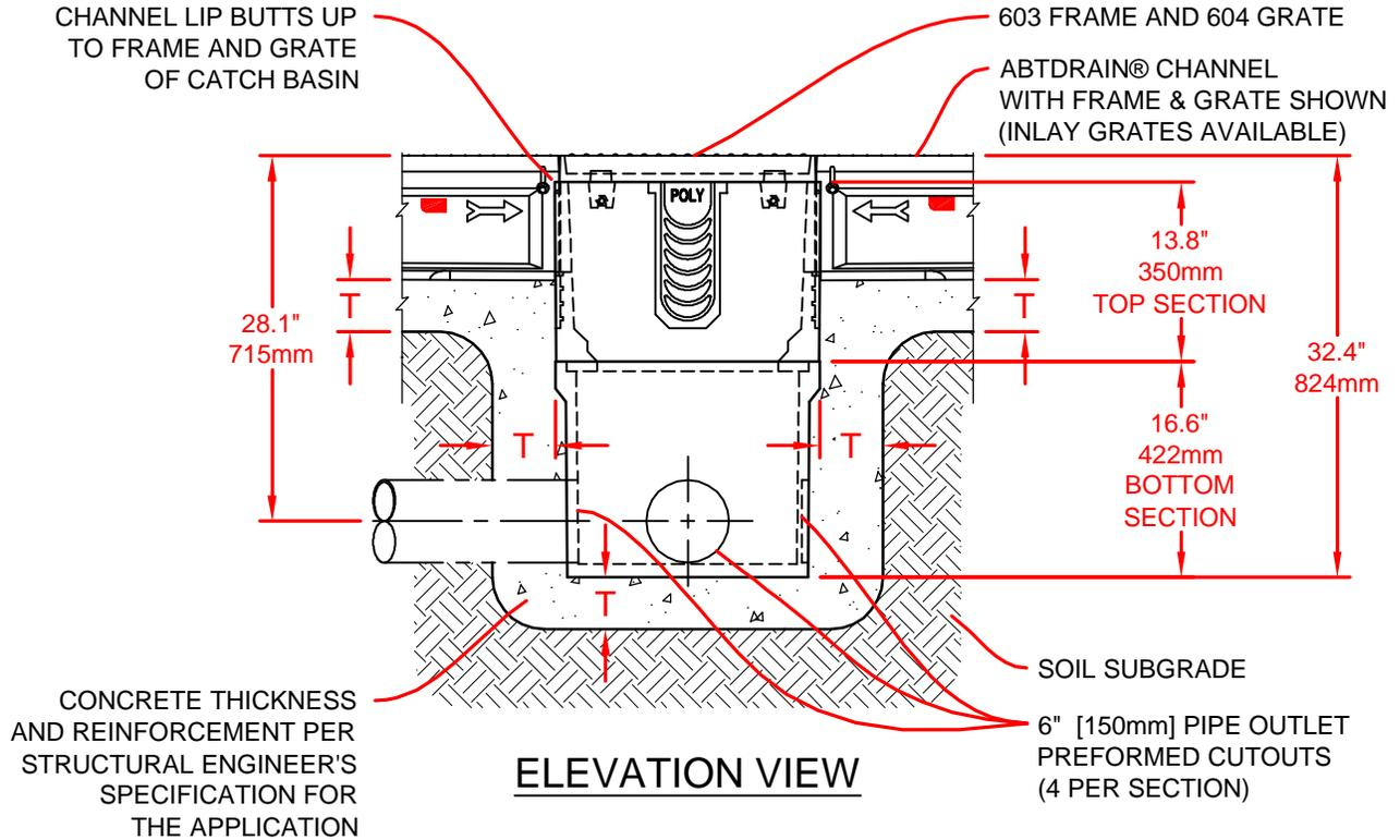
**T** = FLOOR SLAB THICKNESS, OR 4" MIN. [100mm], OR SPECIFICATION (WHICHEVER IS GREATER)
